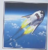
The Dream Chaser<sup>®</sup> is a reusable lifting body spacecraft that can be operated by a pilot or flown autonomously.
